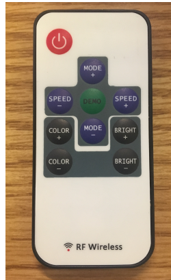
Figure 3: Remote Control for the Noctilux. COLOR+ and COLOR- are for changing colors of the LED. MODE+ and MODE- are for changing the lighting pattern. SPEED+ and SPEED- are for changing the frequency of the repeating lighting patterns.
