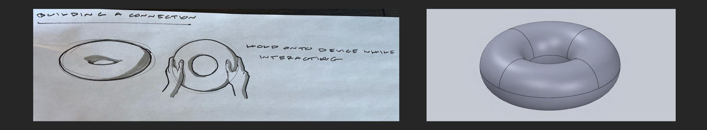
Due to the short nature of the project, minimal form consideration went into the design of my artifact, so a simple form that allowed for successful communication of the desired interaction was chosen. Quick sketches were used to understand form and size, and Solidworks CAD modeling program was used for the digital creation. The model was then imported into Keyshot for rendering of material and context. This process was fairly simple as this was a snapshot of my background in Industrial Design.
