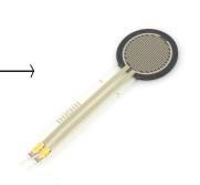
The FSR sensor that is under the pillow triggers all outputs to start once the user lays their head down on the pillow.
