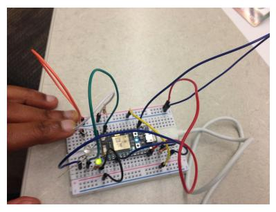
Picture showing circuits response to fridge being open longer than 10 seconds
